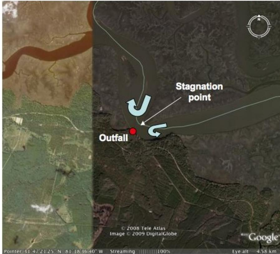
Figure 1: *Secondary circulation eddies generated by ebb and flood flow around a curving channel. The effect is to create a stagnation point that reduces flushing efficiency in the area around the outfall. The image is from Google Earth and shows the location of the outfall Laurel View River.*
