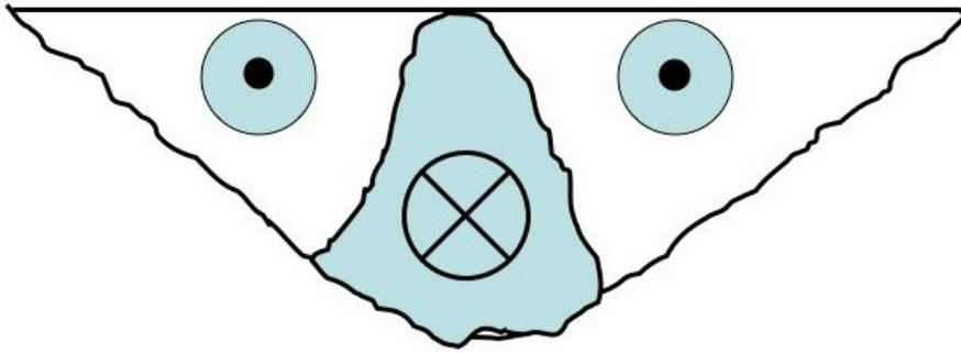
Figure 2: *Hypothetical circulation across a tidal channel showing a net landward flow along the edges (from Li and O'Donnell (2005)). The shaded zone with the "X" in a circle represents flow toward the ocean; the circles with a dot represent landward flow.*
